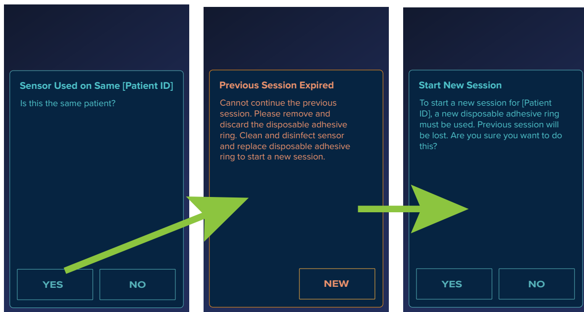
Figure 25. Notification prompts to confirm starting a new session on the same patient if the sensor is still connected to the monitor.
