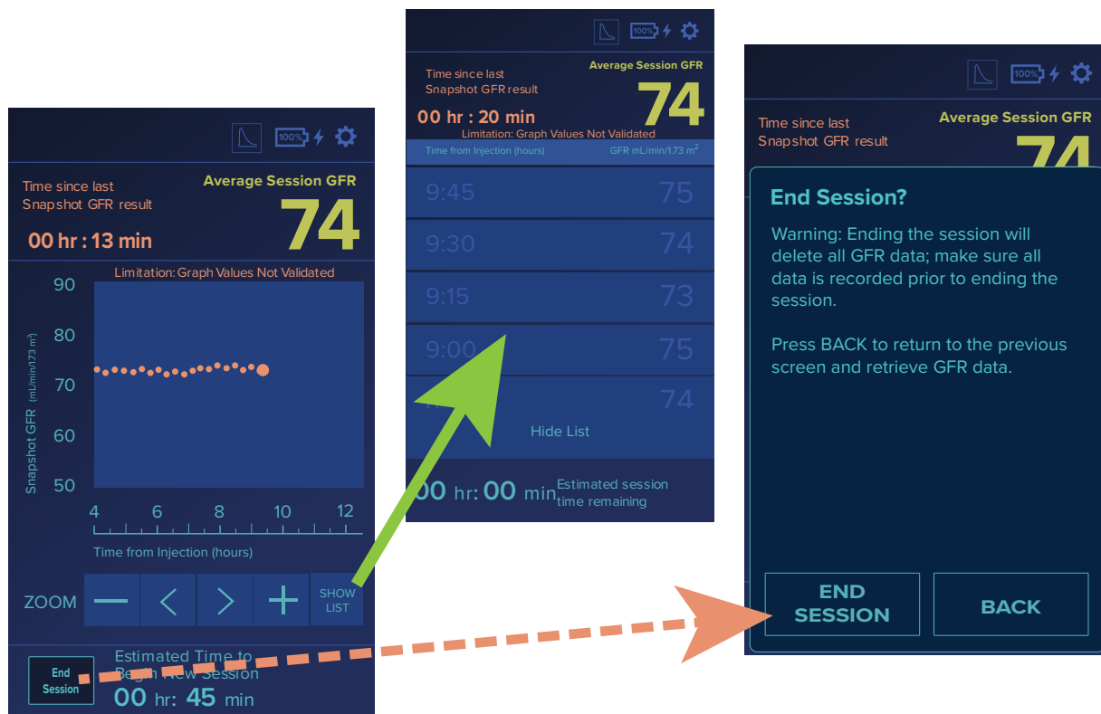
Figure 23. Workflow screens for ending a monitoring session. Press the “SHOW LIST” button to display and manually collect session data (Green Arrow), then return to the ‘End Session’ screen. Press “End Session” button (Orange Dashed Arrow) which will show a confirmation screen. When the Average Session GFR is recorded, press the “END SESSION” button on the confirmation screen.
